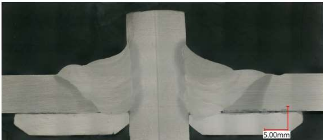
Fig. 2 The macro cross-section is shown after etching to reveal the macrostructure. 10% Nital.
